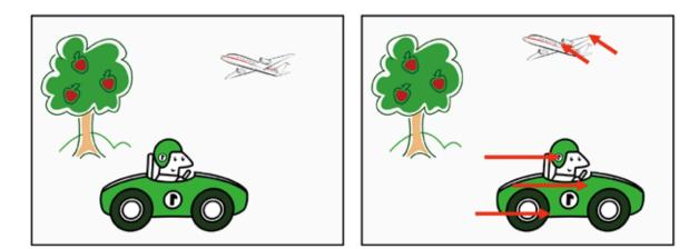
Conceptual diagram showing optical flow. Red arrows indicate motion vectors.
