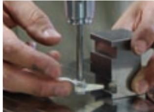
Using a "CeZr Side Measurement Probe for Digimicro" to measure machined dimensions of a transverse groove
