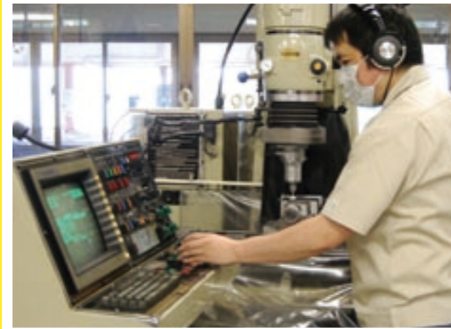
Jig grinder made by Moore Tool of the United States: The operator uses his left hand to carefully control hole dimensions and pitch while aurally checking the grind stone that performs sun-and-planet motions.
