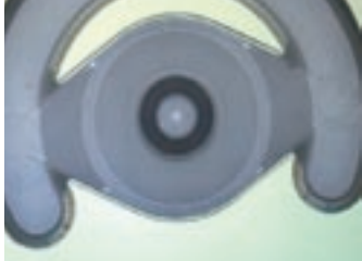
The center hole diameter is 0.11 mm. This hole is where ferrules with runners attached and optical fibers are joined.
