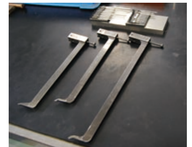
Pin-type probes of various diameters (at back) and probes for horizontal channel measurements (in front)
