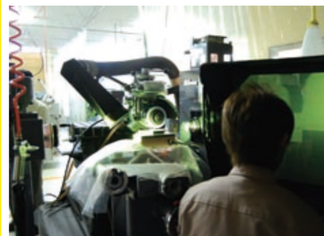
Okamoto Machine Tool Works horizontal optical profile grinding machine with Nippon Kogaku OGC-2 (1973) is in operation to constantly grind profiles.
