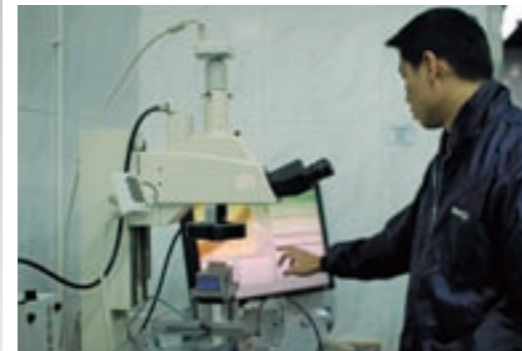
Taking measurements and making calculations with the Nikon MM-60 measuring microscope configured with a high-resolution DS-2Mv digital camera and E-MAX metrology software. Using a large LCD touch screen flat panel instead of a mouse has improved measuring efficiency.
