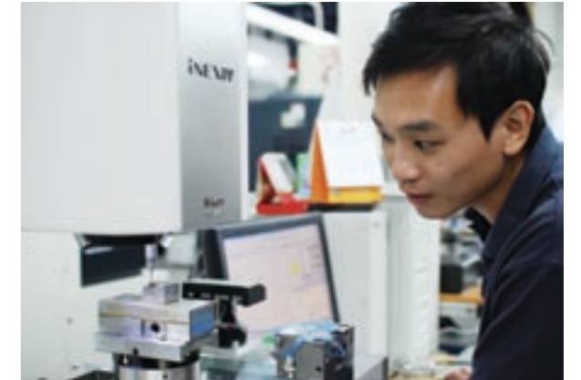
Using the iNEXIV VMA-2520 CNC video measuring system and touch probe to measure the side walls of part
