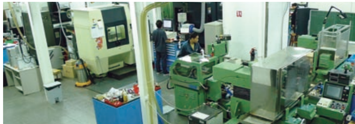
SPH's Tooling Department. The floor has been designed to minimize vibration, and control humidity, temperature and temperature gradients at appropriate levels.
