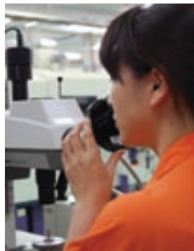
Measuring a rake angle through a 1-minute reading protractor eyepiece
