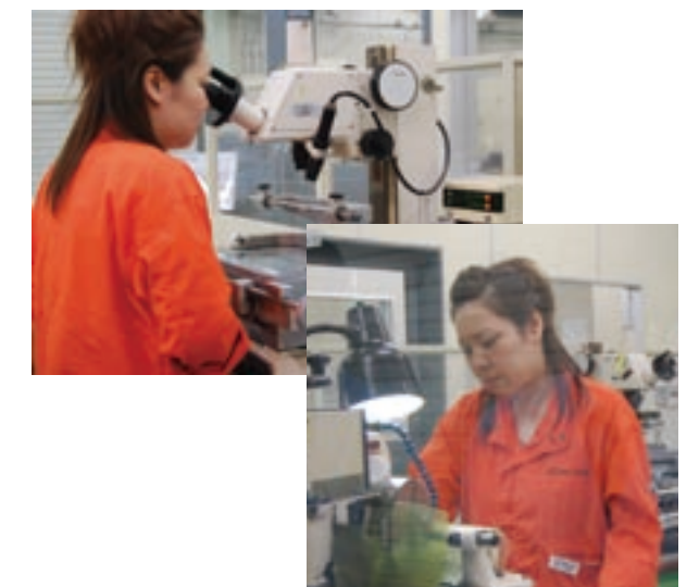
Special blade mounting process: An experienced operator is in charge of both measuring and machining. He can achieve finishing precision of up to 1/1000 mm (1µm).
