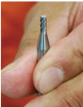
End mill with the tip cut off. The rake angle makes 2D measuring possible.
