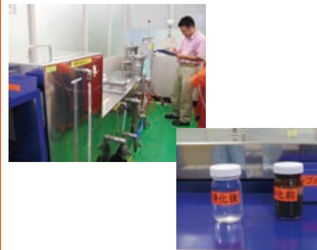
Detergent cleaning system (left photo), and samples comparing before and after cleaning (right photo)
