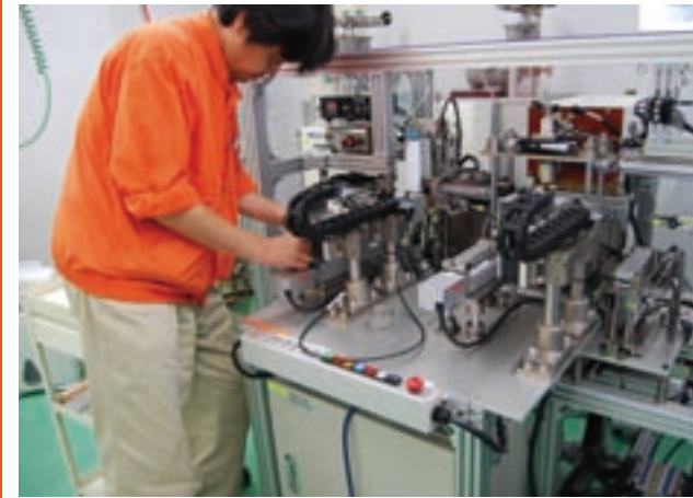
cBN automatic waxing unit developed in-house. NS Tool's unique innovations in machining and inspection processes can be seen everywhere in the plant.
