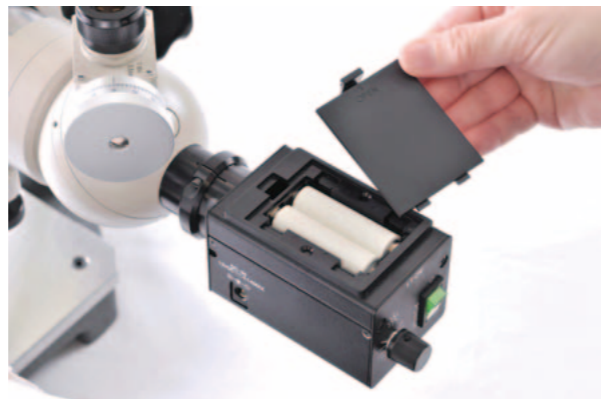
The switch to an LED light source allowed the device to run off two AA batteries. This made the device easier to use and it can still be operated for long periods—even without mains power.
