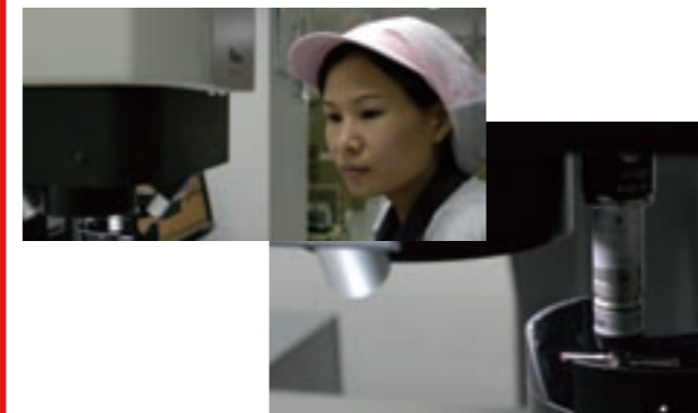
Taking measurements using a Renishaw TP20 touch trigger probe with a star stylus attached to it. During teaching, points to be measured are easier to check by turning on the LED ring illumination.
