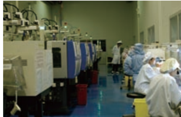
The injection molding line and assembly line in the clean room started operations in 2009. Each part that is formed in the clean room is visually inspected and packaged.
