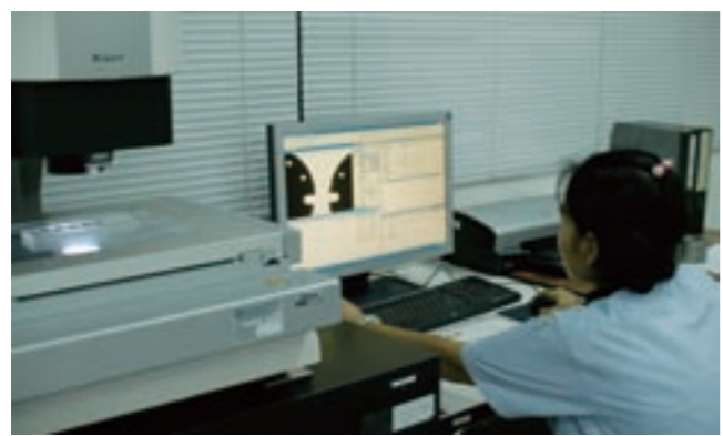
Teaching the positions of multiple samples lined up on the stage. The automatic continuous measurement program using the APS function can be executed by simply designating the approximate start position.
