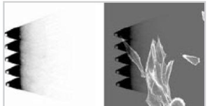
Figure 2: Calibration of LSCM images using the Direct Overlay function.
