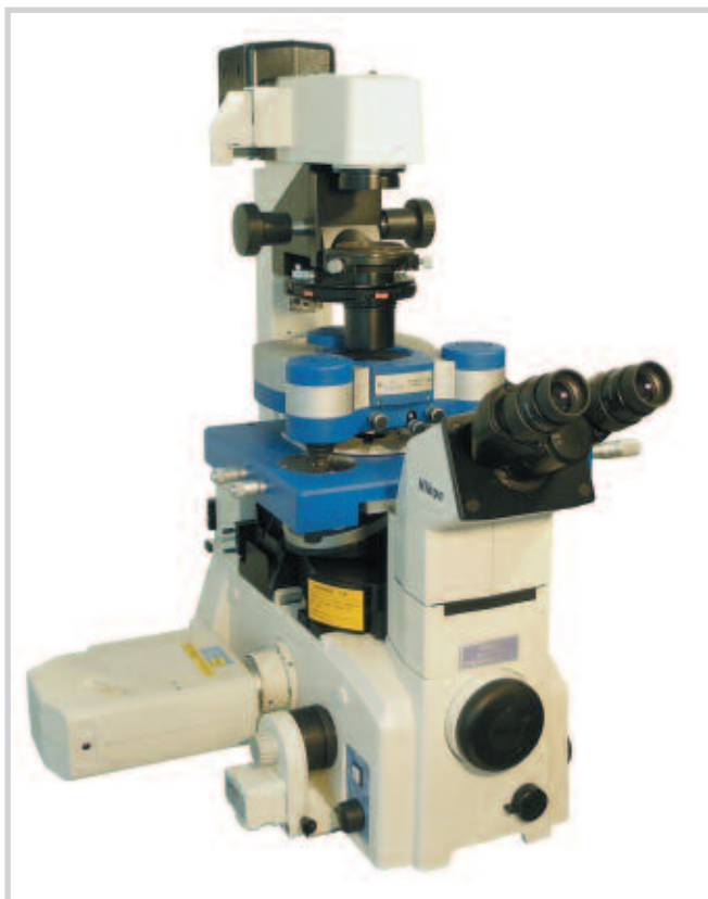
Figure 1: Configuration of the Nikon confocal and JPK AFM on an inverted microscope. Please note that the microscope stage is replaced by the AFM optimized stage for improved stability.
