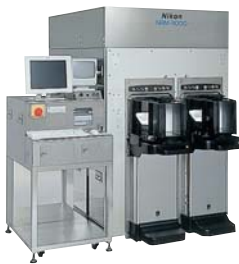
NRM-3000 Overlay measuring system for process management support of 300-mm IC wafers
