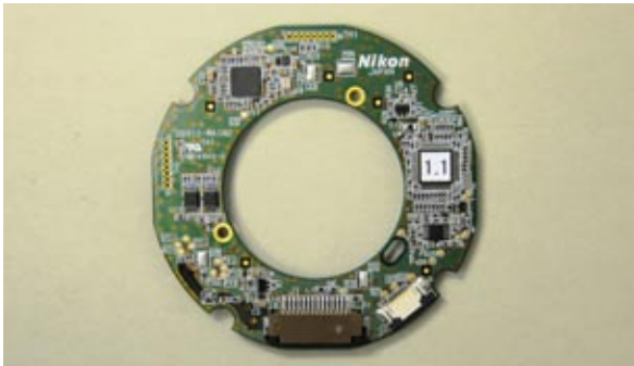
Control board for fieldscopes featuring Nikon's vibration reduction (VR) system
