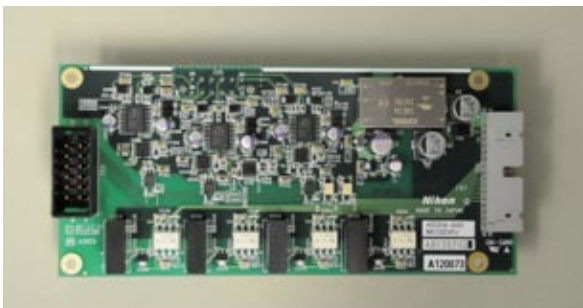
Control board for the latest model ArF immersion scanners
