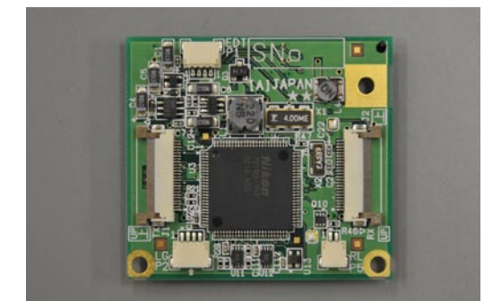
Printed circuit board for land surveying equipment
