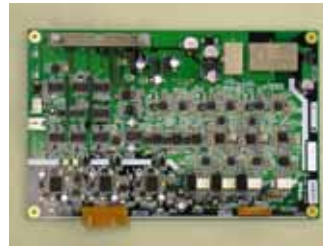
Motor control board for an immersion scanner
