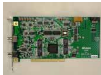
Image processing board for a confocal microscope
