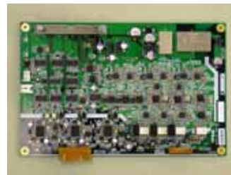
Motor control board for an immersion scanner
