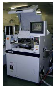
Cream-solder printing machine at Sendai Nikon
