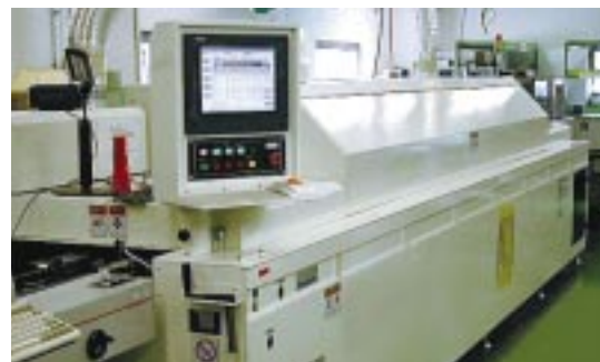
High-performance reflow furnace for lead-free soldering
