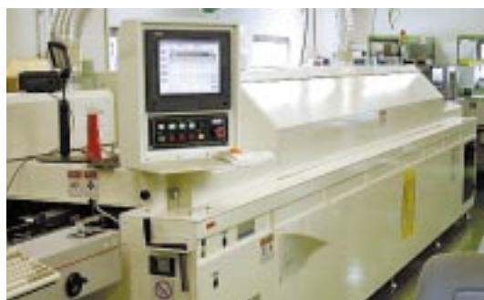
High-performance reflow furnace for lead-free soldering
