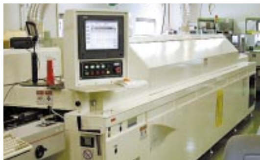
High-performance reflow furnace for lead-free soldering
