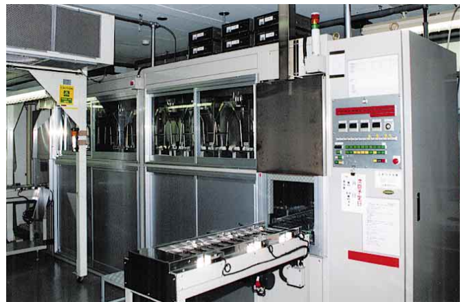
A lens wash finishing system using IPA (isopropyl alcohol) instead of CFCs
