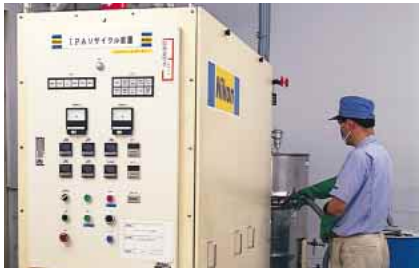
IPA recycling equipment in use at Sagami Plant
